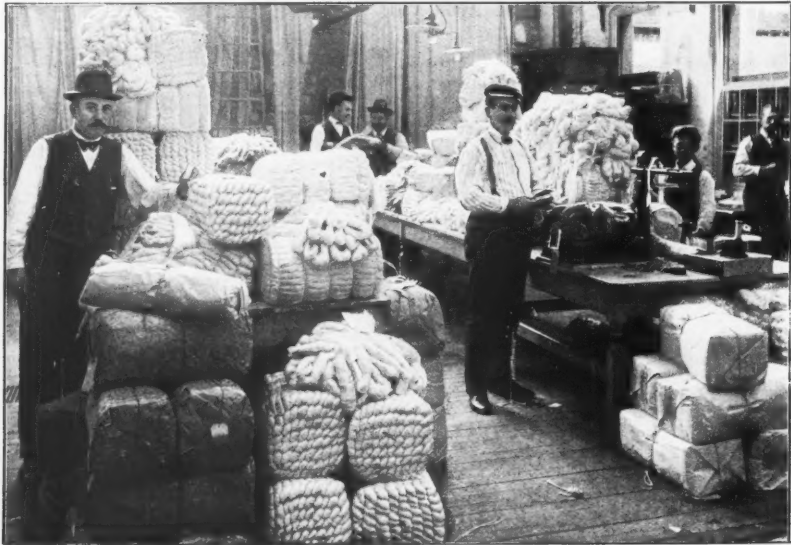
WEIGHING AND LISTING THE SKEINS AS THEY COME FROM THE THROWSTER PREPARATORY TO DYING.
